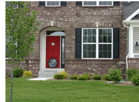
Photo: Ryland Homes blower door test Home Energy Efficiency with HouseWorks®
