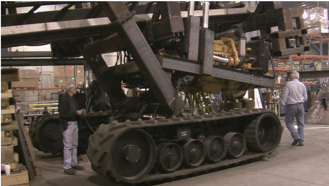
Figure 1. EPS Tree Harvester showing rear tracks and diesel engine (yellow).
