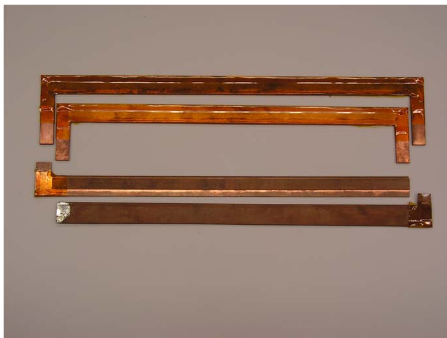
Figure 9-6: 'L' and 'C' Shaped Bars for Rotor Winding
