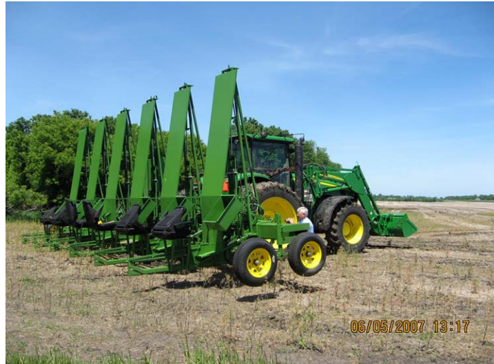
Figure 4: EPS Injection Planter with GPS Guidance System on Tractor 3-Point Hitch
