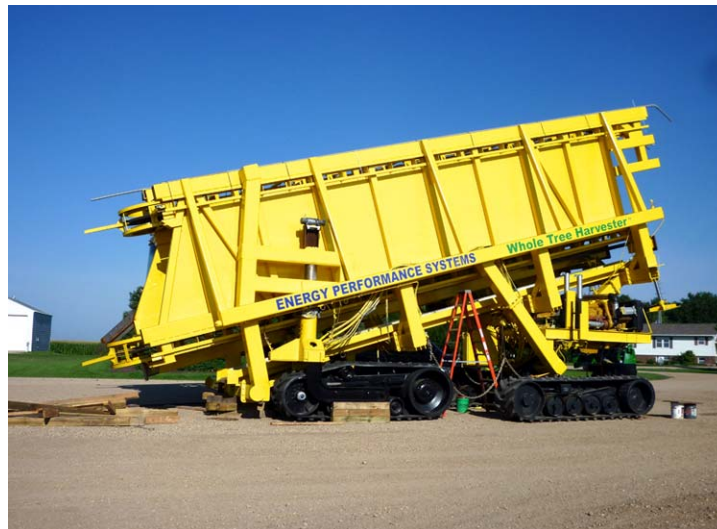
Figure 17: Whole Tree Harvester™ Reassembled Except for the Cutting Blades and Guides
