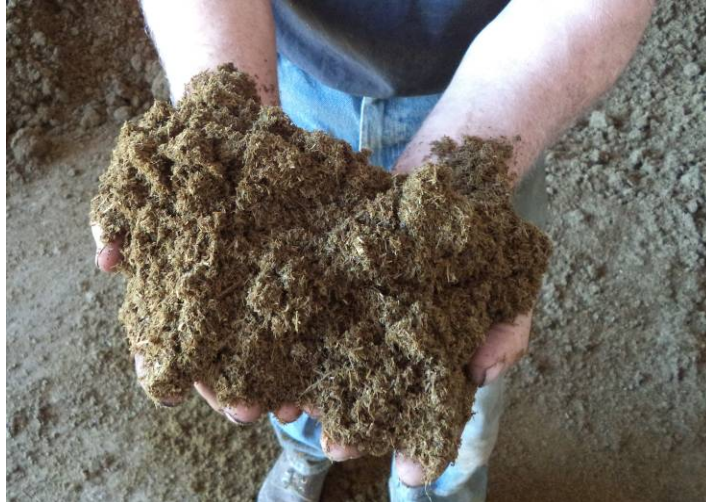
Photo 10: The solid particles separated out of the digested slurry are a soft, sterile and odorless product for use as cattle bedding.
