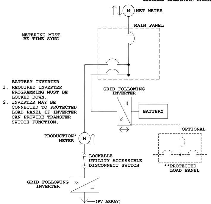
\*3. PRODUCTION METER IS REQUIRED BASED ON THE DER SIZE AND PROGRAM UNDER WHICH THE APPLICATION IS SUBMITTED. SEE THE APPLICABLE TARIFFS.
