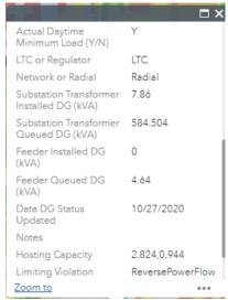
**Network or Radial**: Refers to whether the feeder is laid out in a network or radial fashion.
