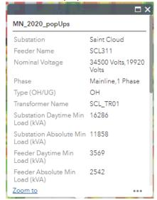
**Substation:** Location where voltage is stepped down from high voltage transmission to a distribution voltage. The conductor system reaching from a substation to the customer is the distribution grid.
