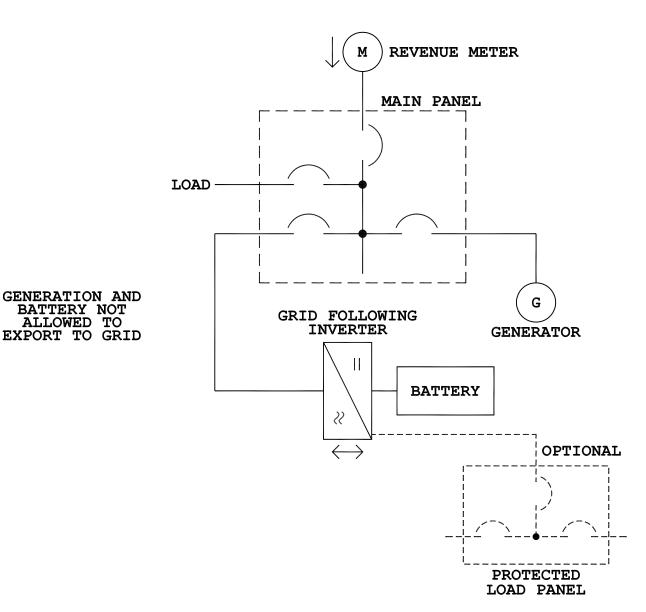
1. THE PROTECTED LOAD PANEL COULD BE A SEPARATE LOAD PANEL AS SHOWN IN THE DIAGRAM OR COULD BE THE ENTIRE MAIN PANEL.
