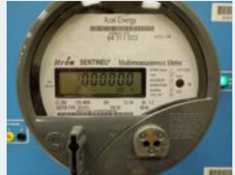
This is a standard meter that determines how many kWh your solar system is producing each month. If you are participating in the Solar\*Rewards program then your production meter will also be used to calculate your monthly Renewable Energy Credits (RECs) payments. The Production meter has a separate account number. The monthly statements are sent to the owner of the PV system.
