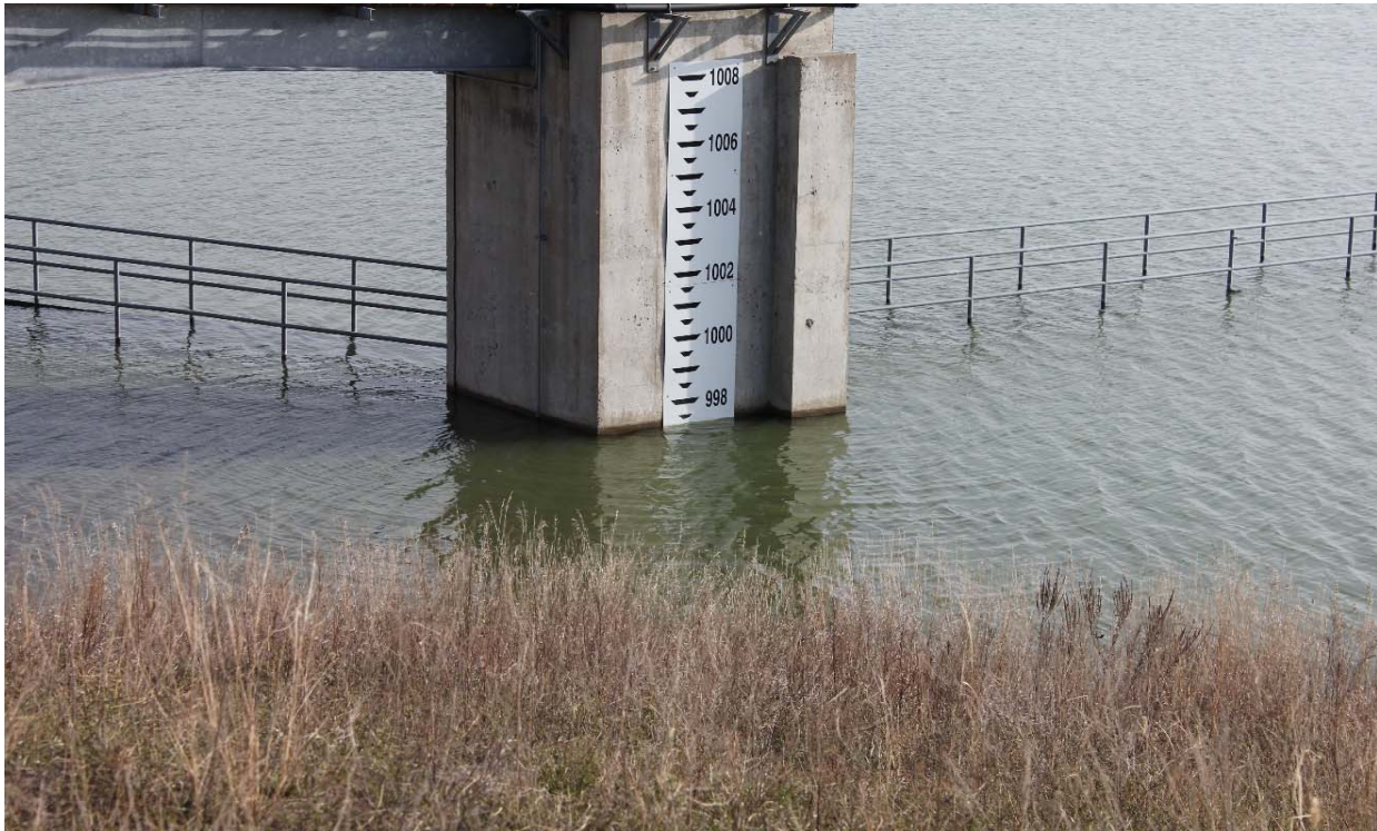
Photo 27 Pond water level staff gauge (shown at approximately 997.1 feet of elevation mean sea level). 11/8/2017
