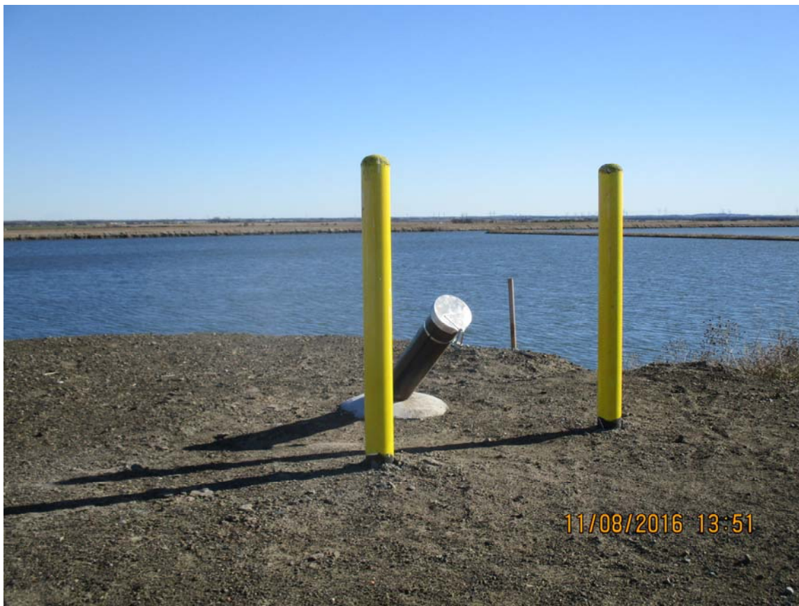
Photo 29 Newly installed pond CCR angled well, looking east
