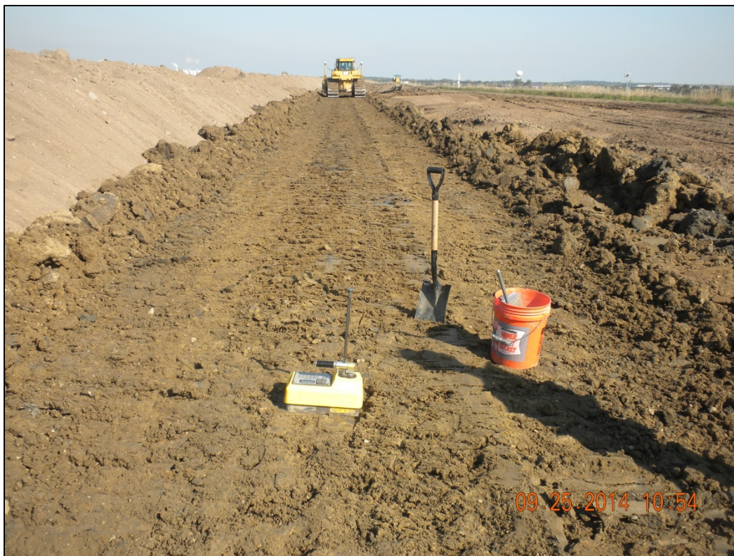
Photo 9: In-Place Clay Density Testing – East Berm Section - Looking North - 9/25/14
