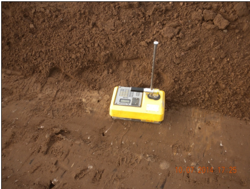
Photo 16: In-Place Controlled cvFill Density Testing – 10/7/14
