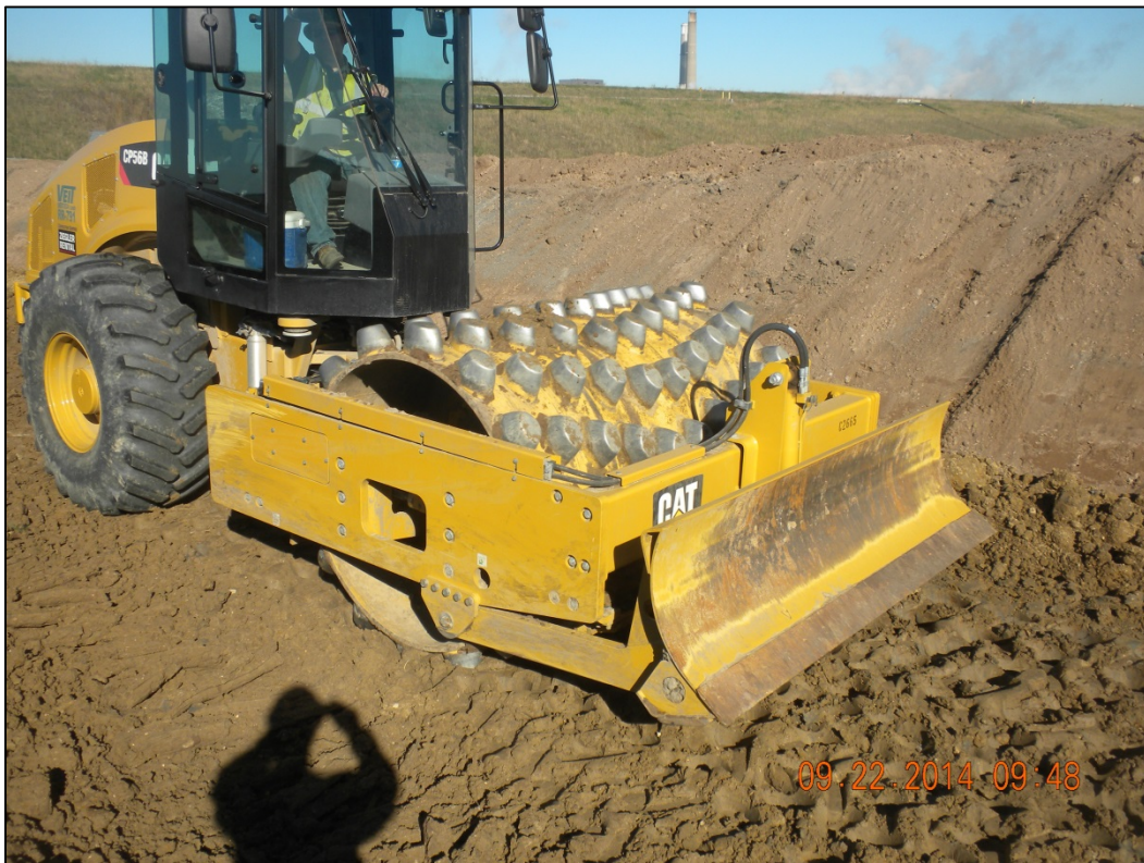
Photo 6: Compacting Placed Clay – South Berm Section – 9/22/14
