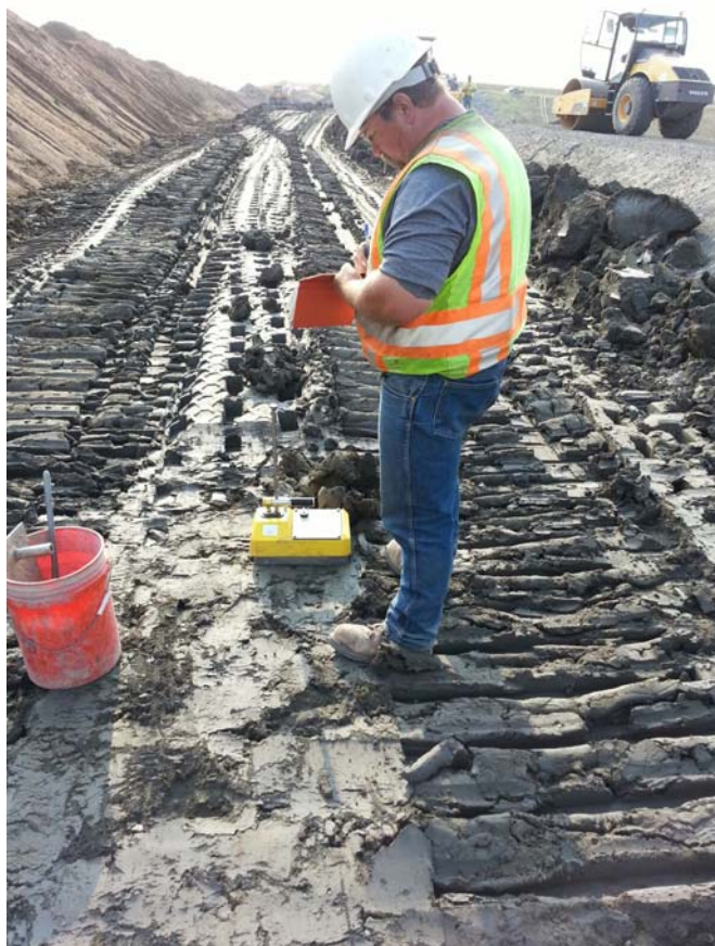
Photo 10 Soil testing technician using nuclear gage to determine clay in-place density and moisture. 8/19/2013
