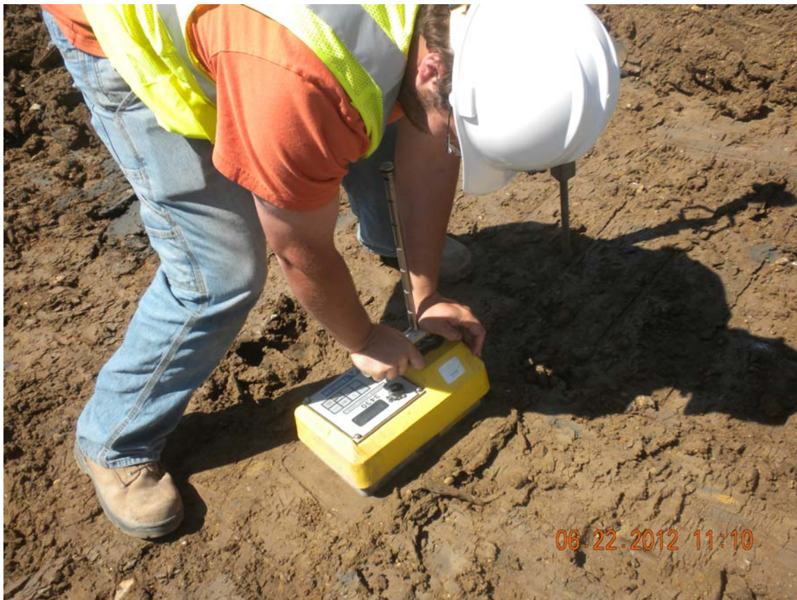
Photo 7 Soil testing technician using nuclear gage used to determine clay in-place density and moisture. 6/22/2012
