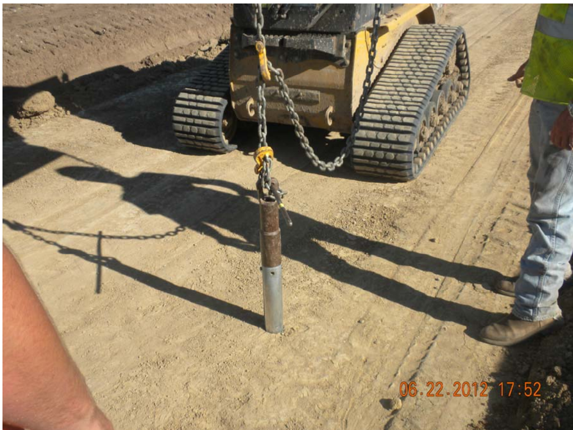
Photo 8 Skidloader extracting thin-wall tube sample to be tested for in-place permeability and index properties. Void created by extracted sample was filled in with granular bentonite. 6/22/2012
