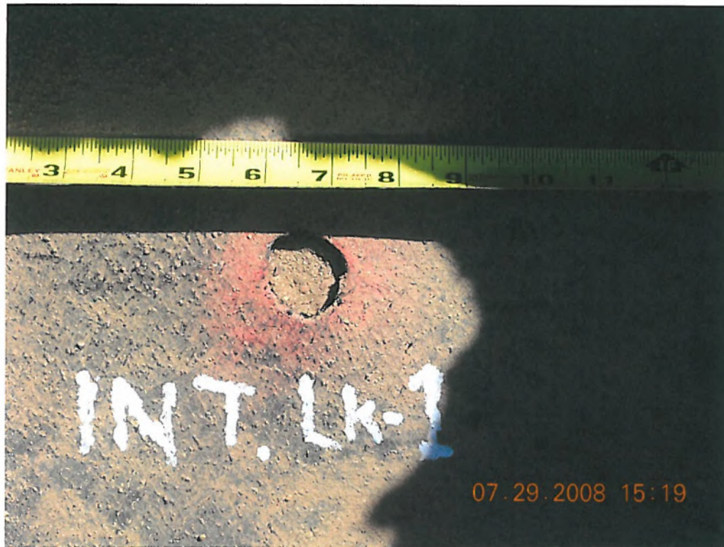
Photo 10: Owner Intentional Leak #1 (penetrating membrane and GCL)
