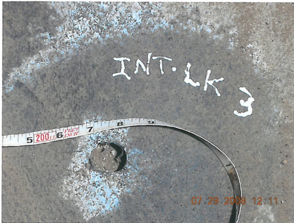
Photograph 12: Owner Intentional Leak #3 (penetrating membrane and GCL)
