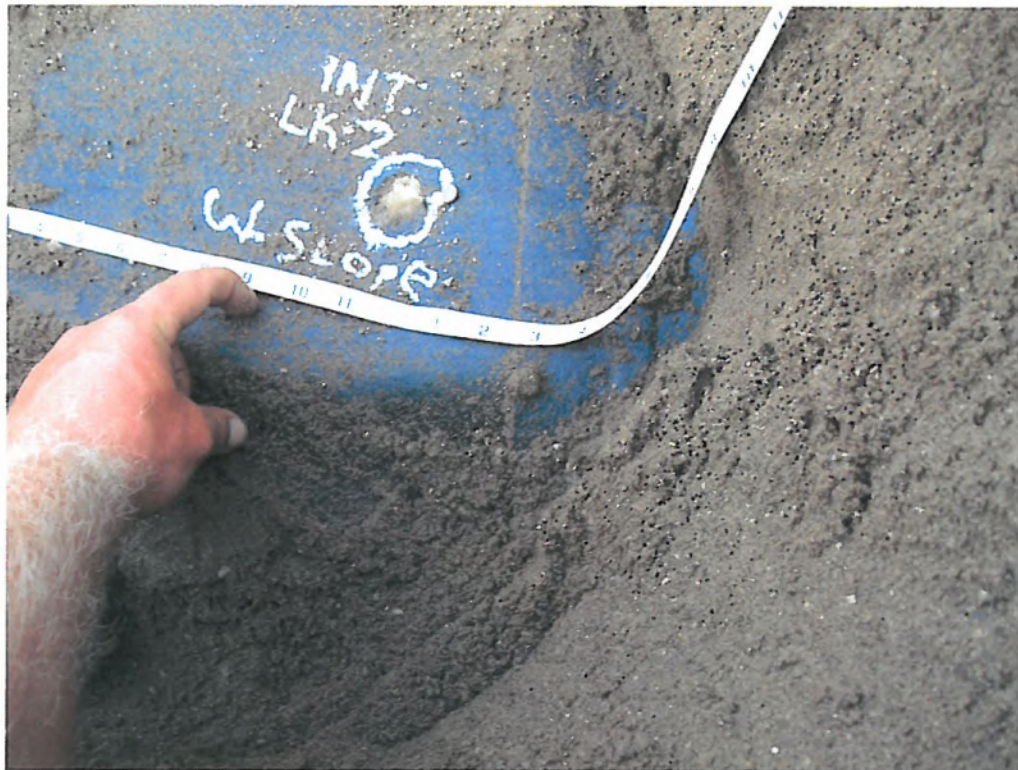
Photo 11: Owner Intentional Leak #2 (1-inch hole through membrane only)
