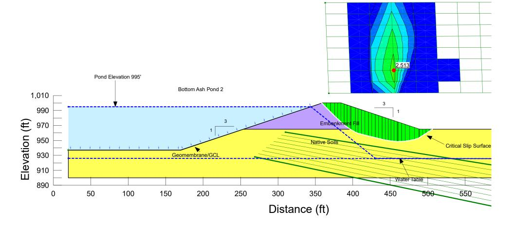
Seismic Condition 3: Maximum Surcharge Northern Dike Critical Cross Section Global Stability Xcel Sherco BAP 2 FS = 2.451
