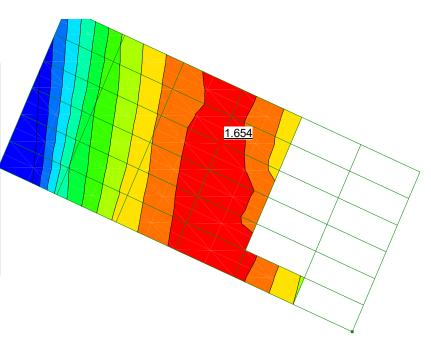
Condition 1: End of Construction Southern Dike Critical Cross Section Global Stability Xcel Sherco BAP 2 FS = 1.654
