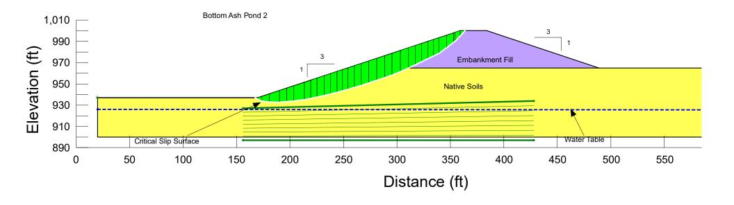
Seismic Condition 1: End of Construction Northern Dike Critical Cross Section Global Stability Xcel Sherco BAP 2 FS = 1.79
