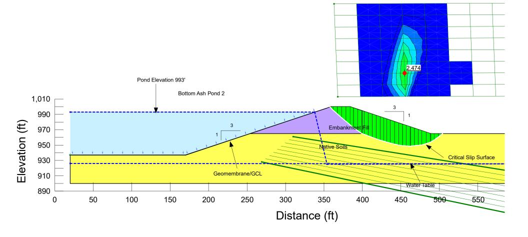
Seismic Condition 2: Max Storage Northern Dike Critical Cross Section Global Stability Xcel Sherco BAP 2 FS = 2.38
