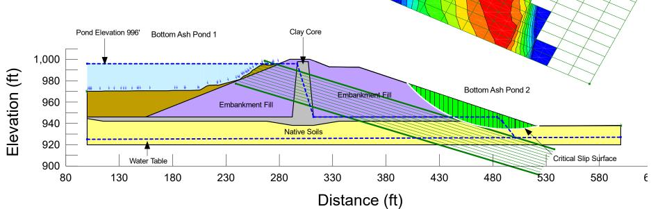
Seismic Condition 1: End of Construction Western Dike Critical Cross Section Global Stability Xcel Sherco BAP 2 FS = 1.616
