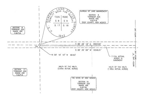
BASIS OF BEARING— Bearings were derived using GPS relative positioning techniques based on an OPUS on September 15, 2014 and are referred to Grid UTM Coordinate System—Zone 13N, NAD (1983).
