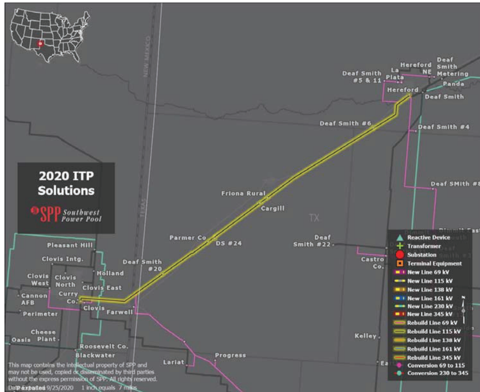
Figure 7.3: Hereford-Curry 115 kV Corridor Rebuild
