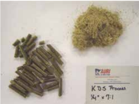
Minnesota Valley Alfalfa Producers—Research to improve pelleting process for biomass to be use as a fuel for an energy facility
