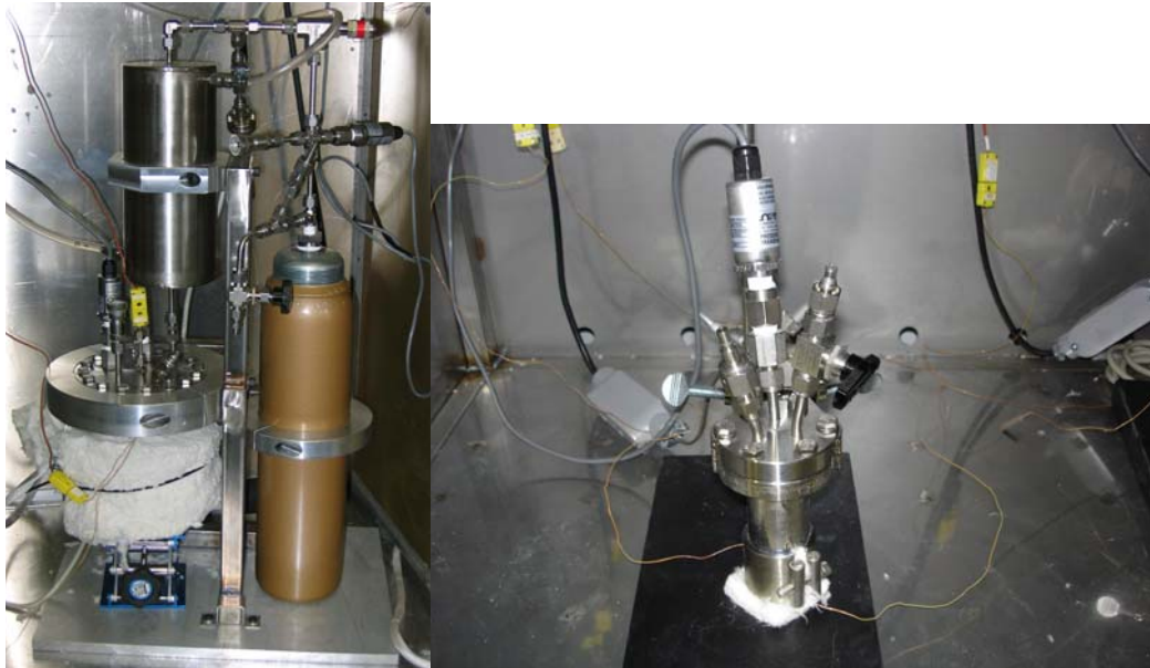
Figure 2: Laboratory batch test reactors: left 1.0 liter with accumulator, right 100 cc reactor
