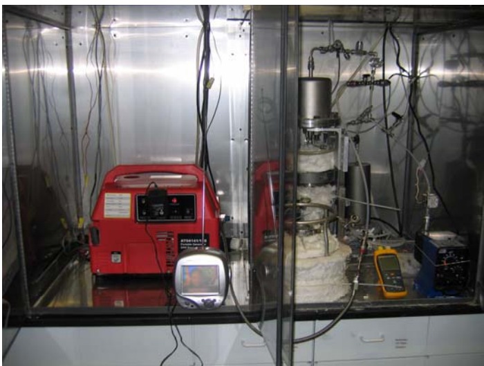
Figure 8: Operation of 100 watts light bulb and portable TV from portable generator fed by hydrogen generated in BFR prototype reformer
