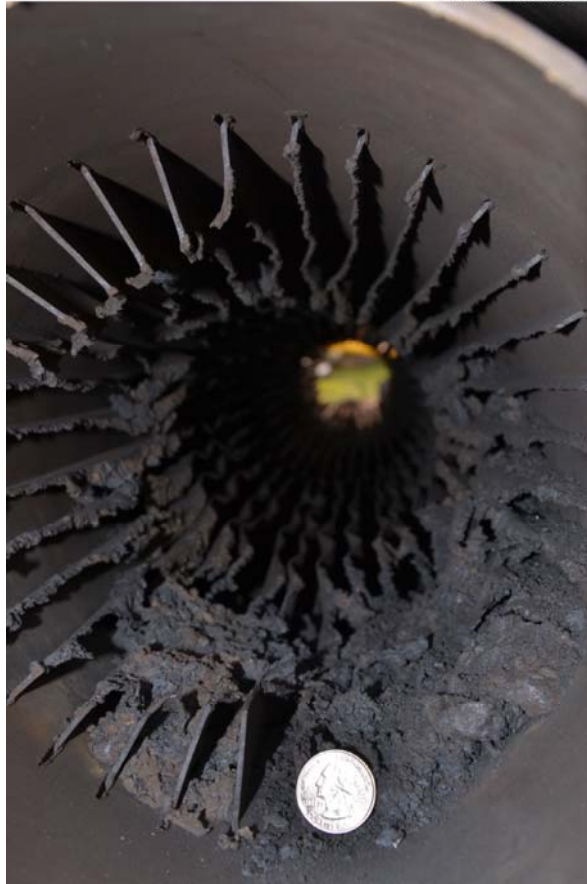
Figure 11. Fin failure due to elevated temperatures at combustor inlet.
